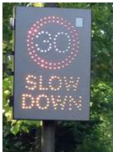
The MVAS sign lights up whenever a vehicle approaches at more than 30mph
